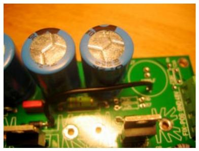
next, connect the anodes of D10 & D13 to the cathodes of D2 & D4:
